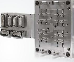
The nozzle wires are run in the channels and protected with the cover plate; this solution keeps the wires from touching the manifold and makes easy to disassemble and sevice.
