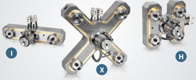
ORYCON's manifolds are built with tubular heating elements embedded in the manifolds heater grooves and covered with swaged –in brass alloy heater covers. This gives the heaters 100% contact with the manifold and therefore optimum heat conductivity, perfect uniformity and long life. Redundant heater elements are another important feature of the Orycon manifold design.
